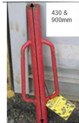
Photo 2 Non-Industrial &/or Shallow Throat Star Picket Driver Not to be used.
