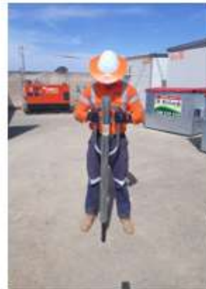
Photo 4 Correct method of using Star Picket Driver, position of hands to remain between waist and shoulder height.
